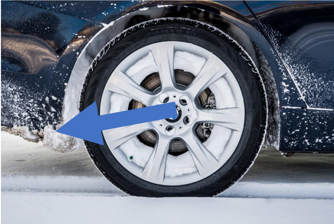
Fig. 1: Slush, packed tight, in a vehicle's wheel arch
